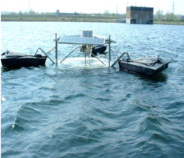
Figure 2. Photo (by V. Lucero) showing one of the SolarBee units operating in EGL4 (the pump station can be seen in the background).
